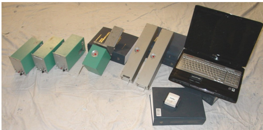
Figure 5: Wave gauges, amplifiers, AD card and PC for wave elevation
